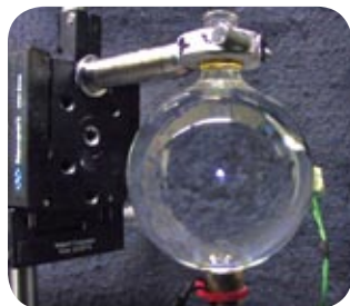
FLASH POINT: In a flask of liquid, a bubble made by sonic waves can collapse to produce light.
